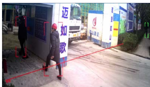
[周界-人员入侵检测]
